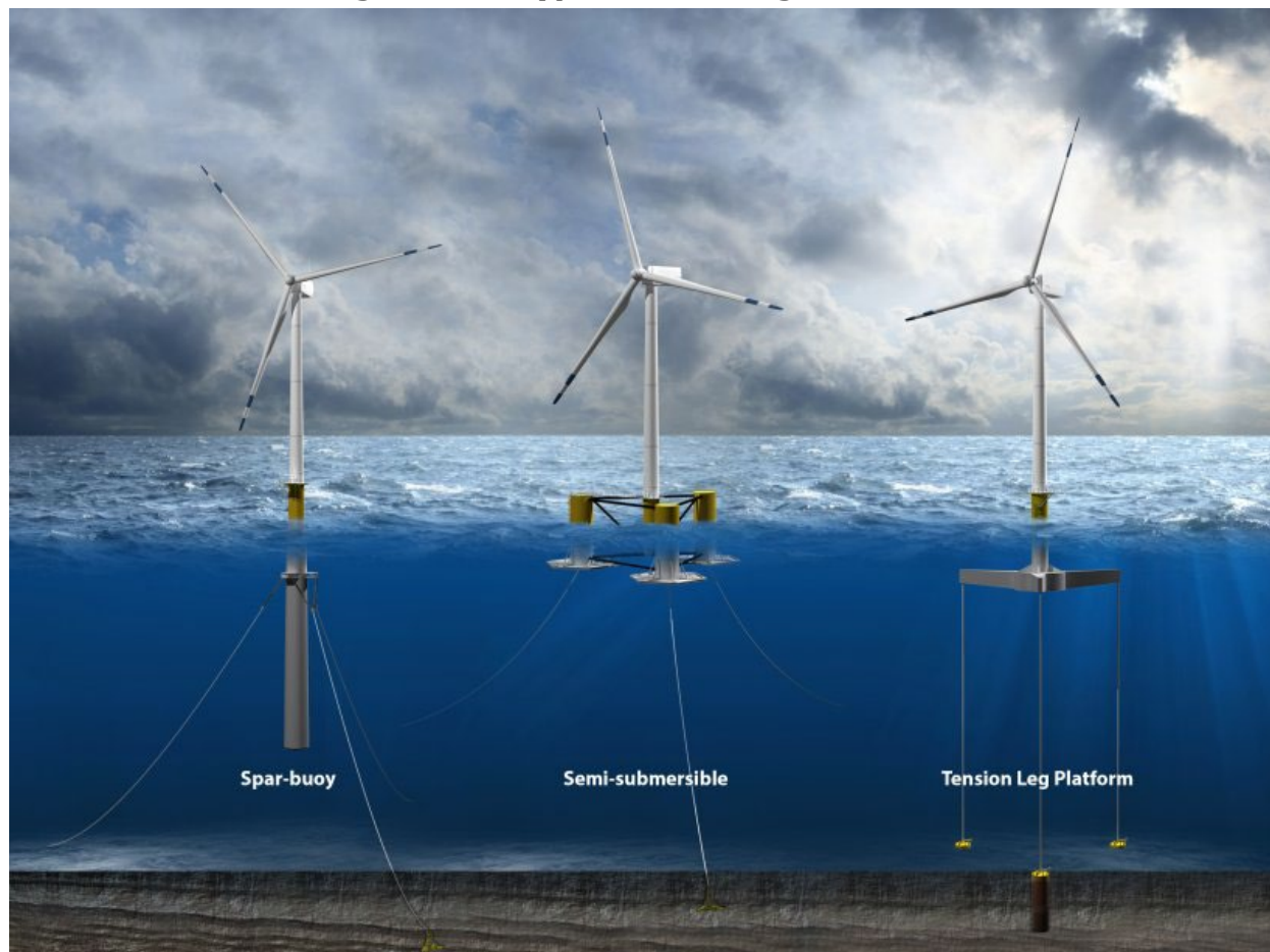
Figure 2-2: Types of Floating Platforms
